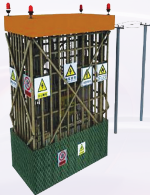
Protection for transformer
